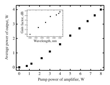
Fig. 6. Experimental results of measurement of average output power versus pump power of amplifier. Insert: experimentally determined spectral dependence of studied GTWave amplifier's gain.
