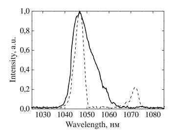
Fig. 4. Spectrum of amplified radiation: dashed line – CW radiation, solid line – pulse radiation.
