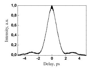
Fig. 5. Autocorrelation function of the amplified pulses (noncollinear scheme of measurements)
