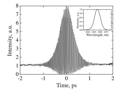
Fig. 2. Autocorrelation function of the pulse intensity of the Yb:KYW laser.
