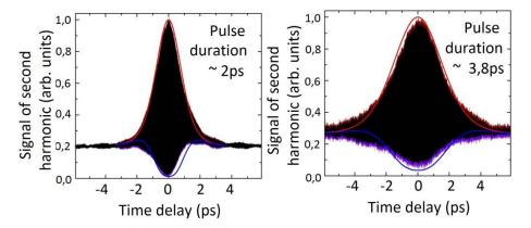
Fig.4 Autocorrelation traces of laser pulses at different lengths of PM-fiber
