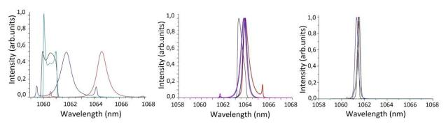
Fig.3 Emission spectra of Yb mode-locked fiber laser for different lengths of PM-fibers and different settings of polarization controller.
