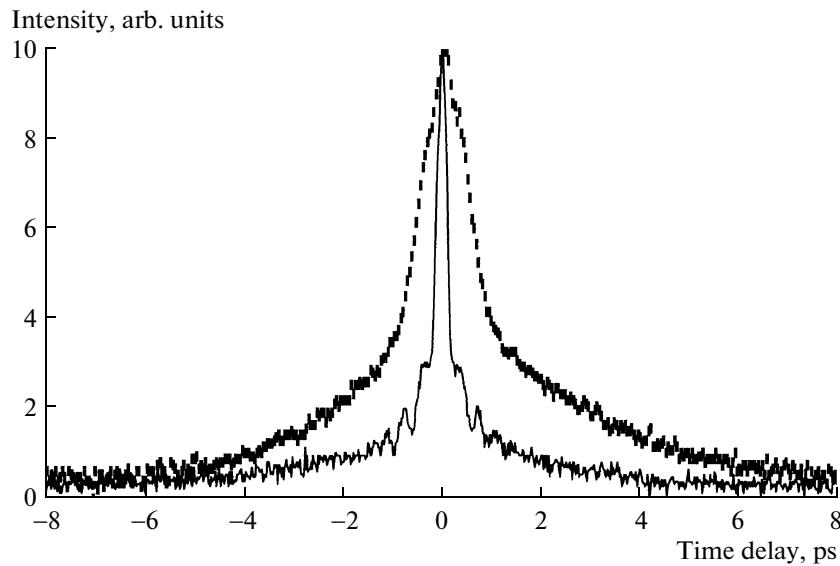
**Fig. 2.** Noncollinear autocorrelation functions of the femtosecond all-fiber ring ytterbium laser: (dashed line) output pulse and (solid line) compressed pulse.
