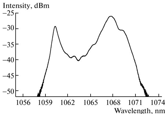
**Fig. 3.** Spectrum of the radiation of the femtosecond all-fiber ring ytterbium laser.
