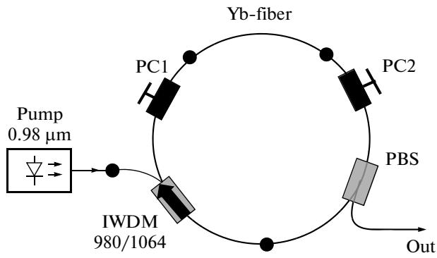
**Fig. 1.** Scheme of the femtosecond all-fiber ring ytterbium laser: IWDM wavelength-division multiplexer and isolator, PC1 and PC2 polarization controllers, and PBS polarization beam splitter.
